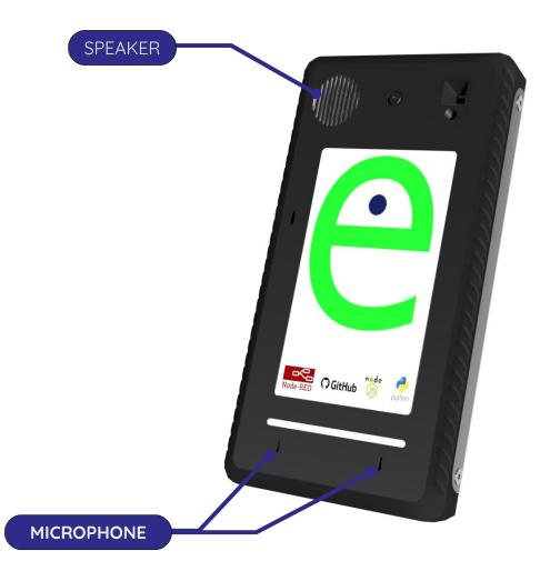
The displaced arrangement helps reduce echoing.
