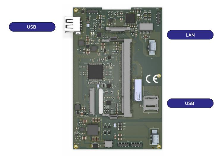
The LAN interface is connected to the CONNECTOR MODULE (on which there is an RJ45 connector) through the 10-pin connector. Of the two USB interfaces, the first is exposed outside, of the system; while the second is internal and allows you to equip the system with a small bluethooth or WIFI device.
