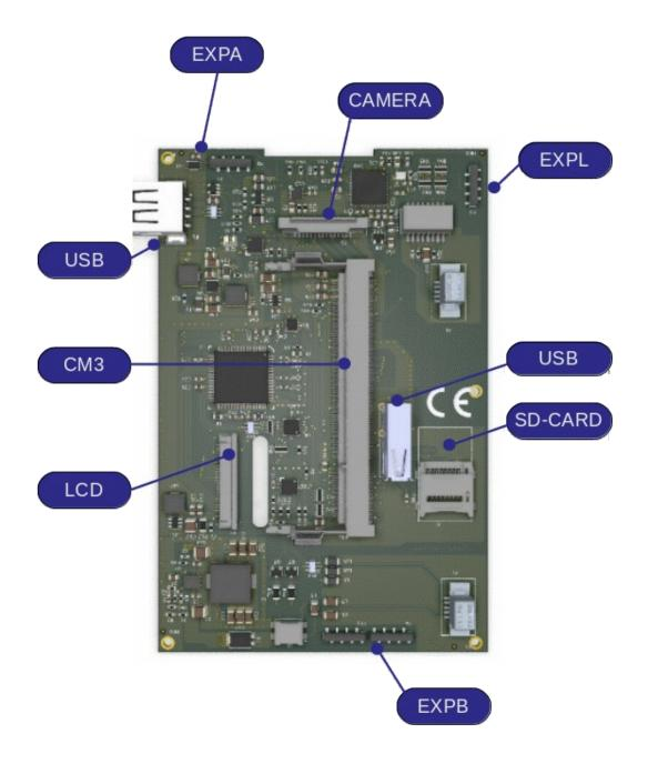
The base module consists of a main board on which the Raspberry CM3 module is installed and equipped with a series of functions and sensors that are fundamental for the functioning of the system.
