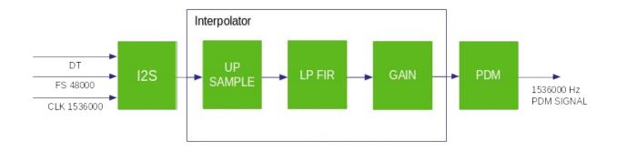
The system operates with an internal DSP frequency of 36,840,000 Hz and supports on the I<sup>2</sup>S side a symbol frequency of 48,000Hz which with two 16bit channels corresponds to a bit rate of 1,536,000 Hz.
