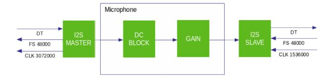
The microphone used is a **SPH0645LM4H-1 MEMS** microphone with 32-bit I2S interface of which 24 are actually used.
